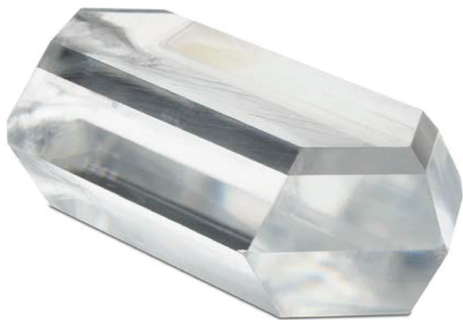
Example crystal boule of KAP grown at Inrad Optics.
