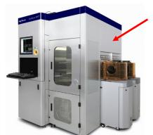
Large, extreme precision optics for semiconductor wafer inspection
