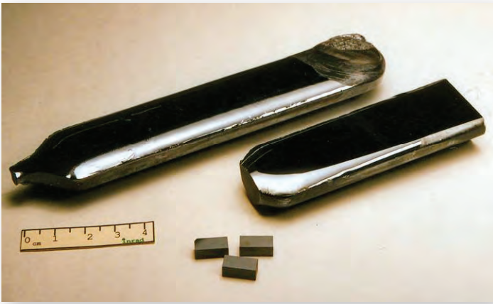
Examples of crystalline ingots of ZGP along with oriented OPO blanks.
