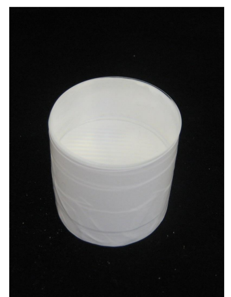
Cylinder wrapped in PTFE tape with a fused silica output window
