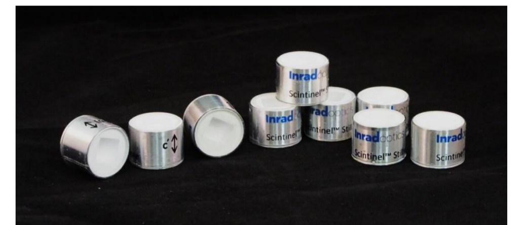
10mm stilbene cubes mounted in aluminum housings, crystallographic orientation indicated for anisotropy studies
