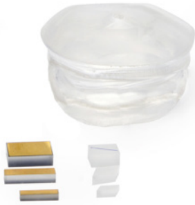
As-grown BBO boule with finished crystals for EO and NLO applications
