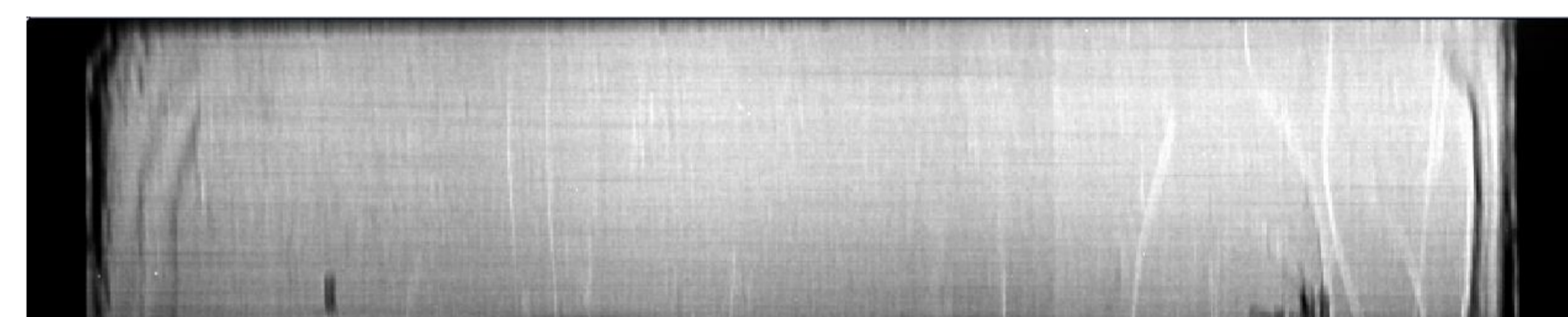
Topographic Image (70 mm width x 13 mm) Resulting From Processing and Stitching Quartz (10-10) Orientation
