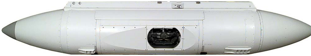
Figure 6. F-9120 installed into AARS Pod for carriage on an F-16C/D aircraft. (Note rotating window center section which provides unobscured horizon to horizon cross track field of regard.)
